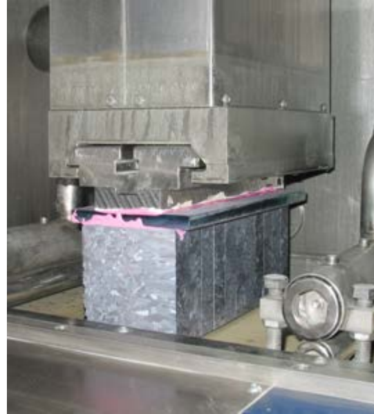
Experimentelle Wafersäge (MWSS)
